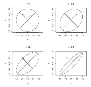
Although the length (eigen values) of the axes differ, their orientation (eigen vectors) are the same.
